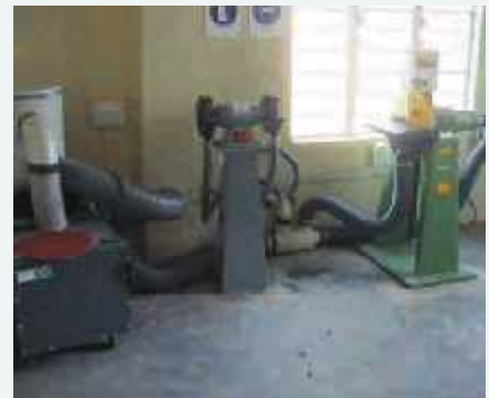
Machine Room with centralised dust extractor
