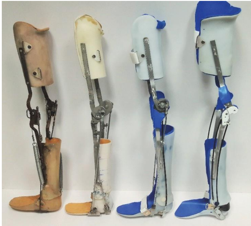
Successive prototypes of mechanically actuated stance controlled KAFO
