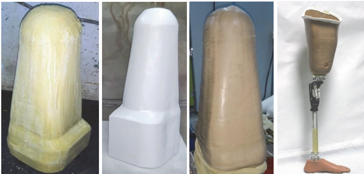
Machined PU stump; resin coat; HDPE socket; prosthesis with knee joint
